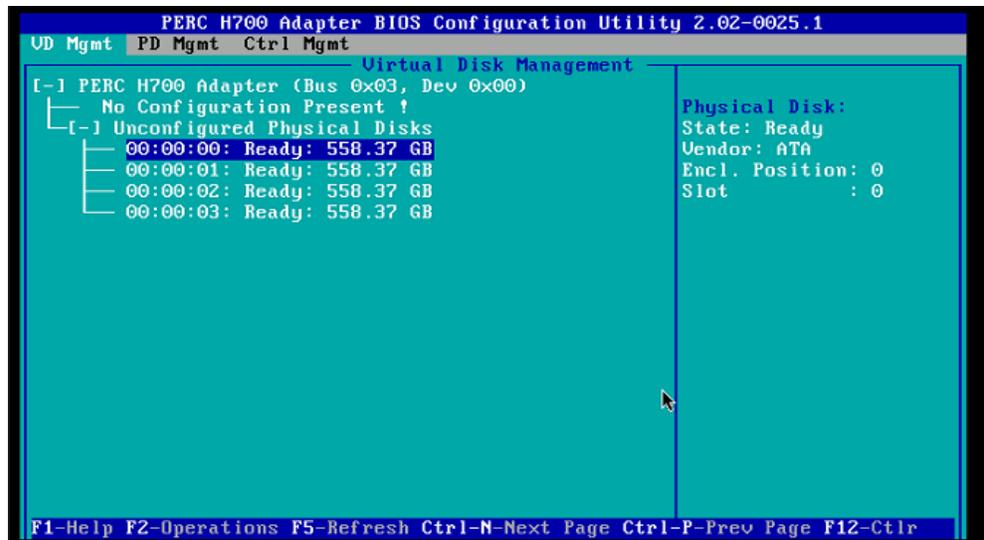
Figure 2-2 BIOS Configuration Utility: Virtual Disk Management
